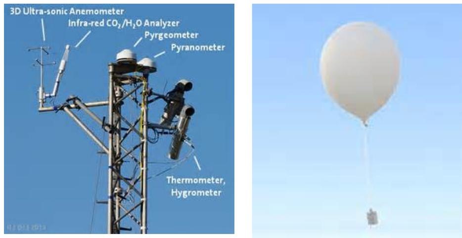
**Figure 4-7 Meteorological instrumentation**
