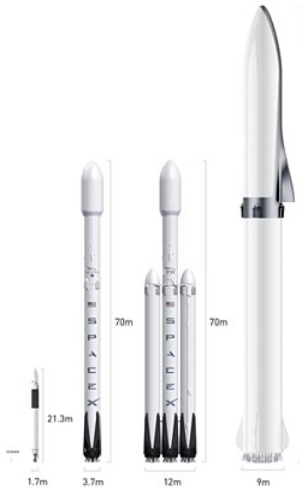
Fig.4. Vehicle overview: Falcon 1, Falcon 9, Falcon Heavy and BFR
