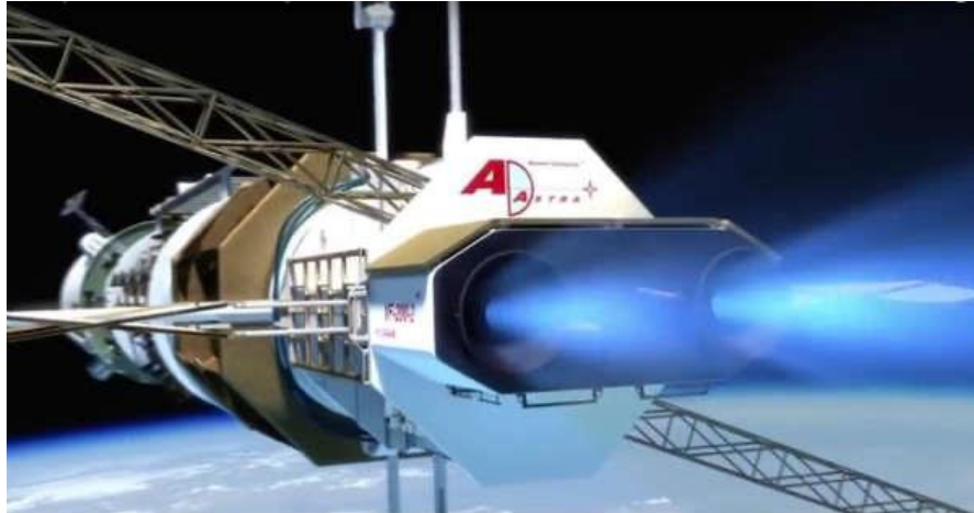
Figure 7.10: NASA's VASIMR Plasma Engine [bing, 2022]
